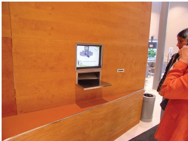
As a patron feeds a returned item into the slot it is automatically scanned and checked in, and a receipt is delivered through the small slot to the right of the return. On the other side of this wall, is a device that pre-sorts the returns into four to six general categories. [SLIDE 013]
