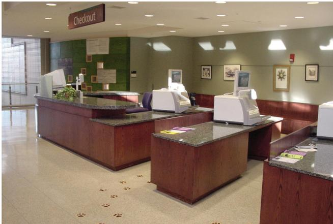
Here, the charging function is on the left as a patron enters the building, so that it's on the right as the patron exits. If the patron wishes to check anything out, they move into one of four aisles, out of the path of others leaving the library, they complete their transactions, and then rejoin the flow of traffic leaving the building.
